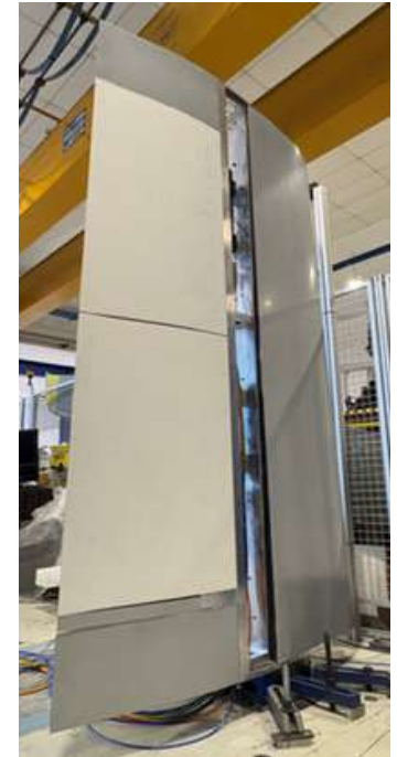
Full-scale morphing aileron structure installed on the dummy wing box designed and manufactured by HAI
