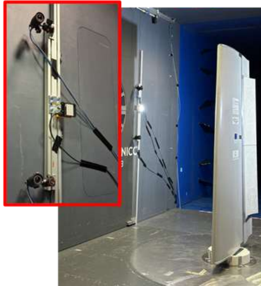
DIC measurements by SIEMENS
