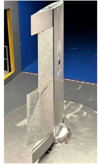
Servo-actuated morphing ailerons
