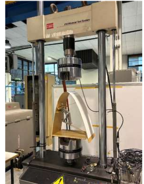
Morphing droop nose demonstrator installed on the MTS universal testing machine for cyclic fatigue testing.
