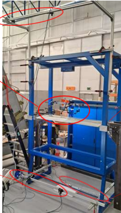
Load cells, Morphing actuation loads
